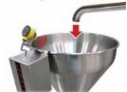
Photo Sensor monitors product level in the hopper and controls the pump
