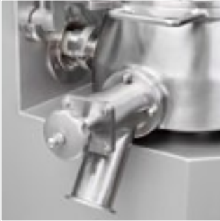
Discharge valve, chopper coupling and safety switch.
