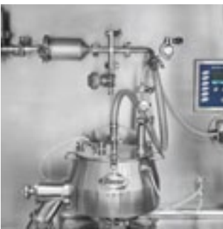
Detail Isolator Installation with vacuum drying.
