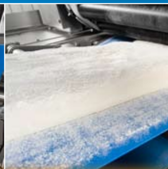
Infeed of the dough sheet reduction
