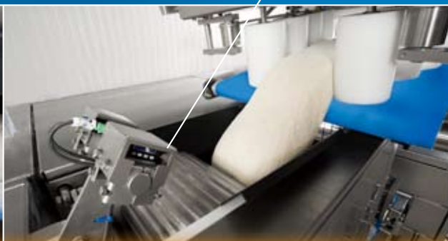
Two sensors control a continuous stress-less dough flow from the dough supply conveyor with dough guiding rollers into the 'Dough Driemer'.
