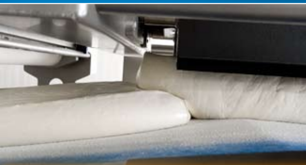
Dough chunks are dropped on top of each other to create a continuous dough flow.
