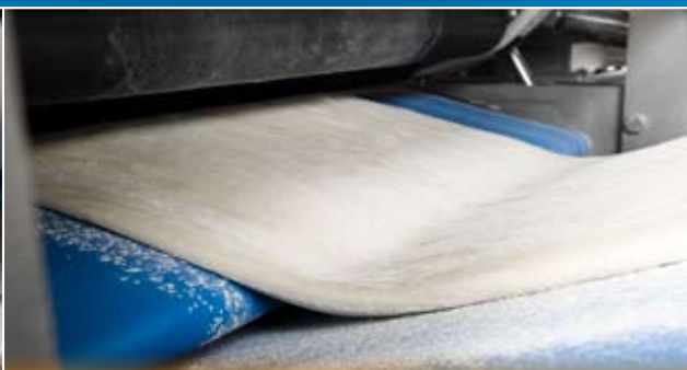
Stress free production due to preventing dropping heights from one conveyor to the next.
