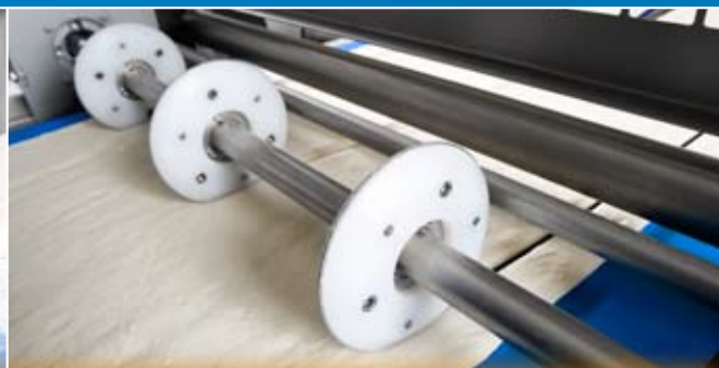
Driven circular cutters. Easy to change over for other products.
