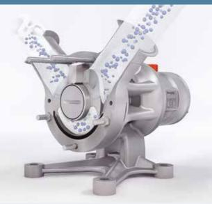
A single sinusoidal rotor creates four evenly sized chambers. As each chamber rotates it gently conveys the fluid from the inlet port to the outlet port. At the same time, the opposite chamber opens to draw in more fluid, resulting in a smooth flow with virtually no pulsation.
