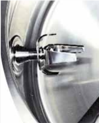
Because of its ideal design and location the chopper tool works effectively even when the mixer is only 30% filled.
