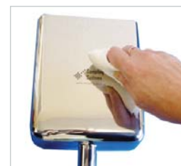
4. Clean etching area thoroughly using demineralised water
