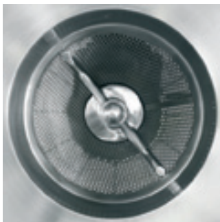
The material can be calibrated during discharge by a sieving mill below the outlet.
