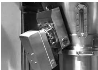
NIR sensor on fluid bed
