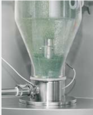
Wurster-Bottom-Spray: Coating in the MINILAB.
