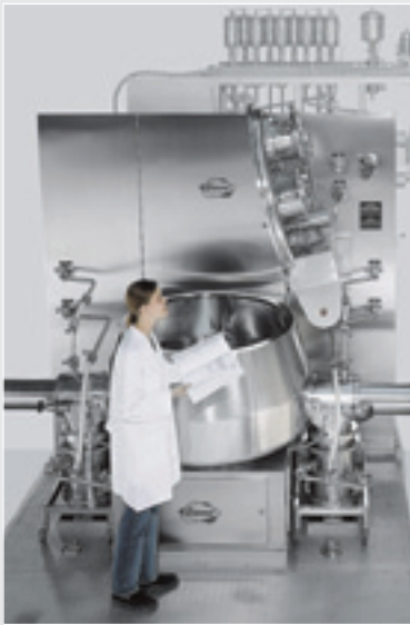
P 600 in modular design, CIP ready, for processing of highly active substances.
