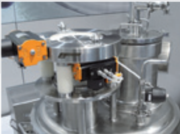
Containment design of mixer lid with split butterfly valve.
