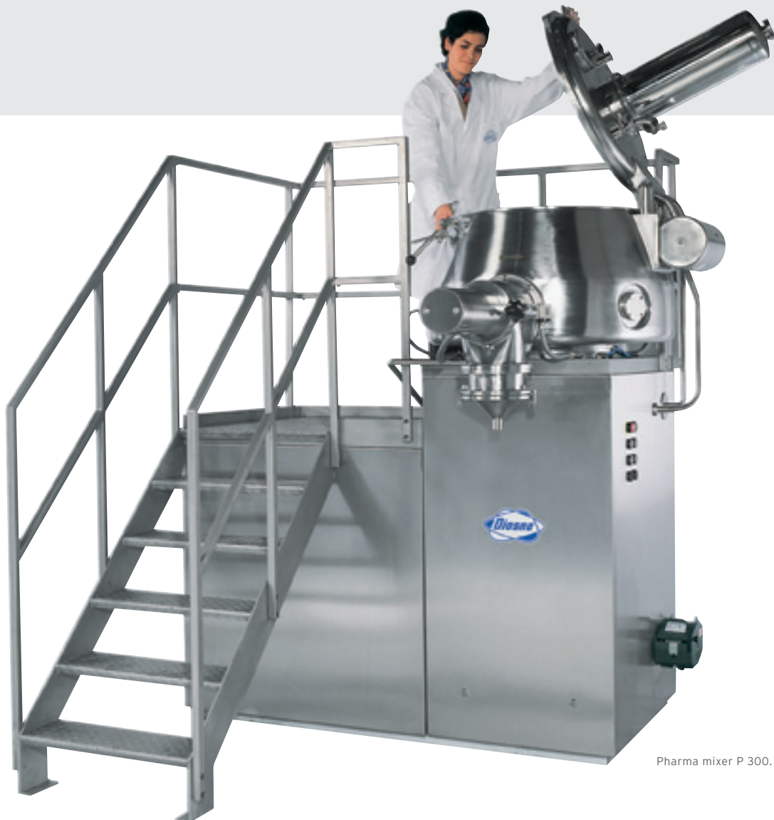
P 600 in modular design, CIP ready, for processing of highly active substances.
