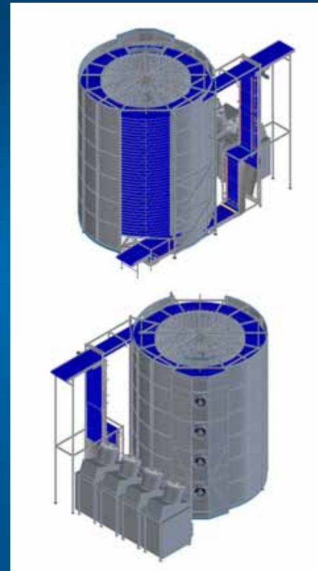
Horizontal air distribution through a spiral tower
