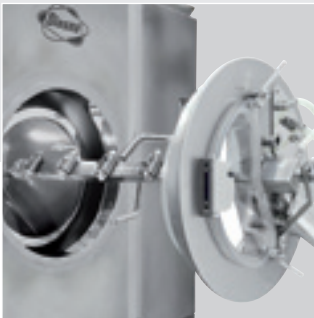
Simple operation due to horizontal removal of spraying device and lid.
